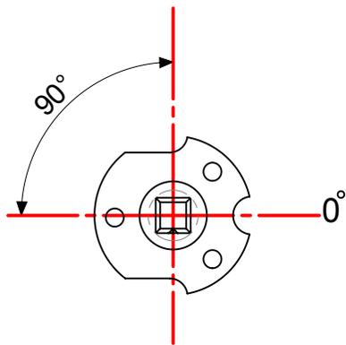
**FIG.01:** FISSARE IL PIASTRINO FISSO ( 1 ) AL BATTENTE CON LE VITI FORNITE ( A ) RISPETTANDO LO SCHEMA "Sc.01" E TENENDO LA SCANALATURA VERSO IL BASSO COME INDICATO.
